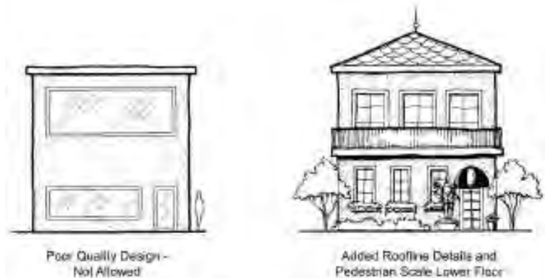
Figure 28. Typical Commercial Design Detail
