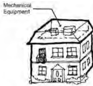
Figure 12. Example of Screening Rooftop Equipment
