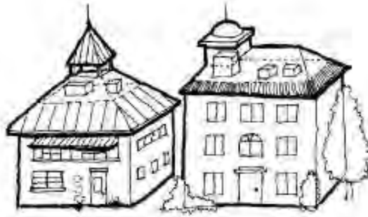
Figure 29. Examples of Screening Mechanical Equipment
