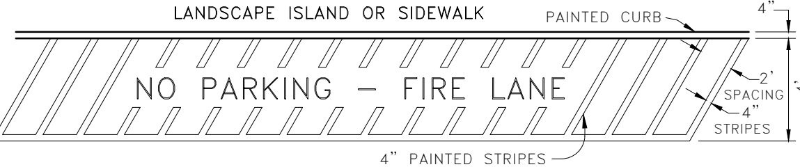
FIRE LANE STRIPING
