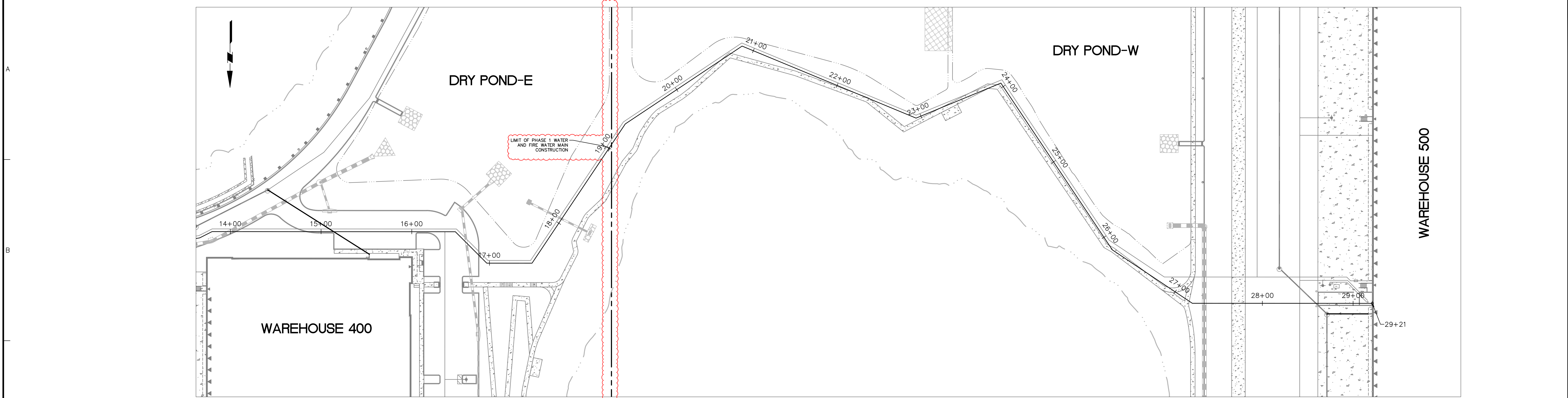
FIRE WATER MAIN LINE-D PLAN VIEW
