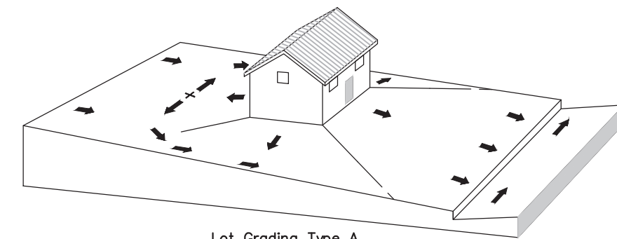
Lot Grading Type A Drainage Directed Toward Front of Building
