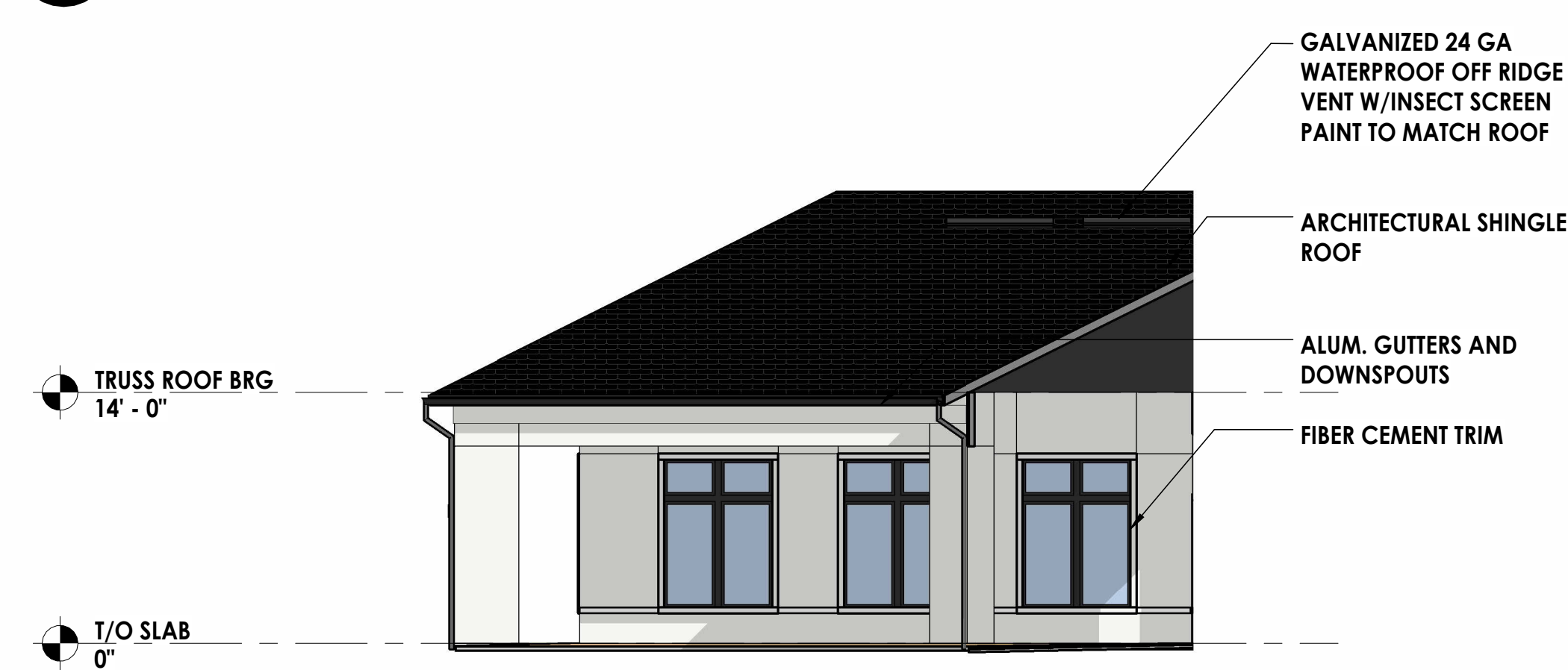
6 RIGHT COURTYARD ELEVATION
