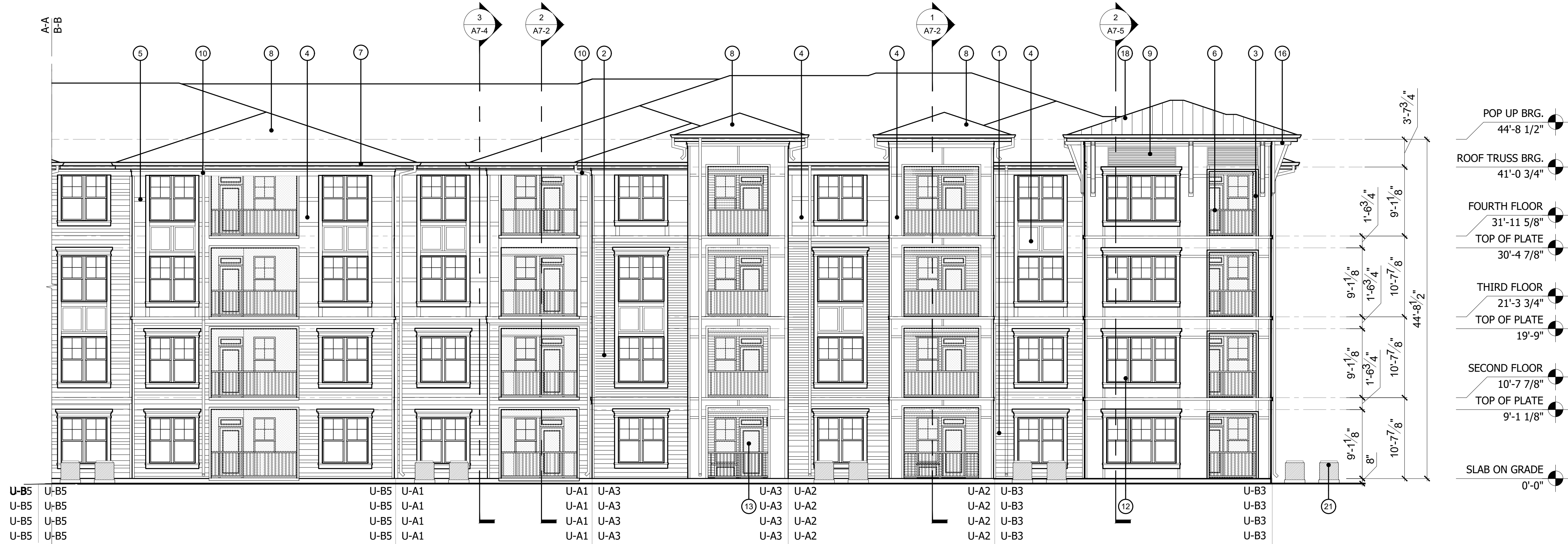
2 A5-1.3 BUILDING TYPE I REAR ELEVATION (A) 1/8"=1'-0"
