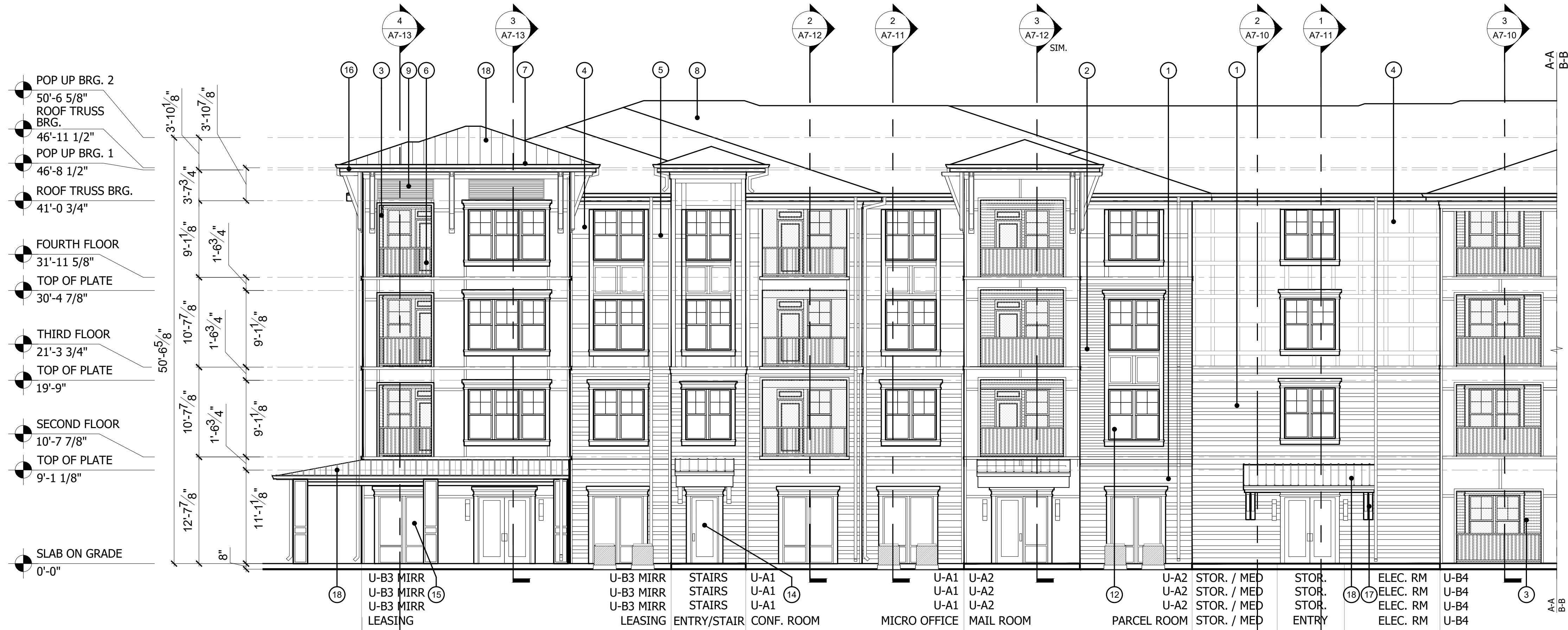
1 A5-2.1 BUILDING TYPE II FRONT ELEVATION (A) 1/8"=1'-0"
